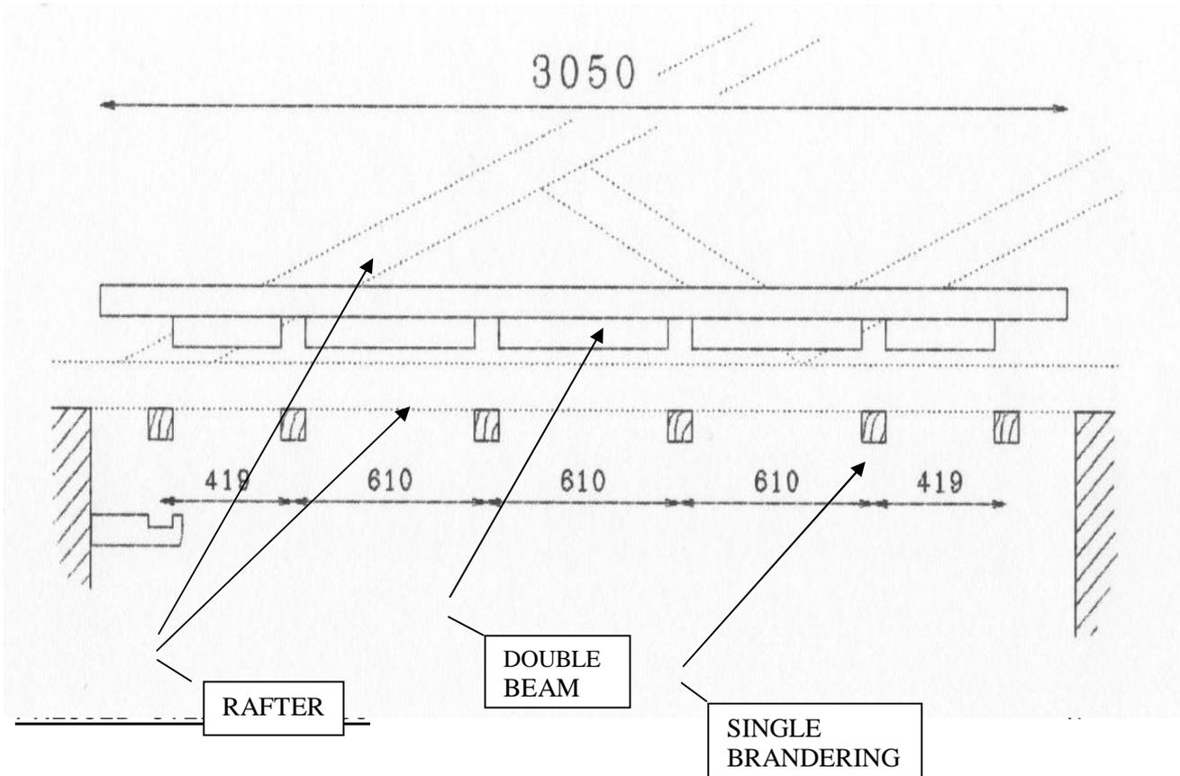
It is important to remember that the screws (or nails) must be placed **“off set”** at the crossing points of the centre lines of the brandering.
