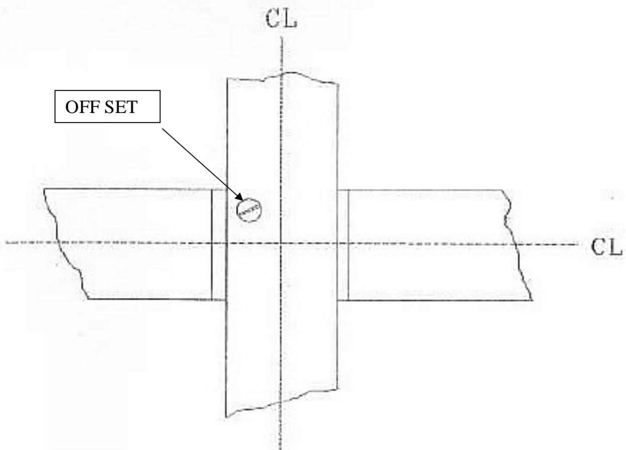
This is due to the fact that the nails holding the plates up will eventually be on the exact crossover point of the two centre lines.
