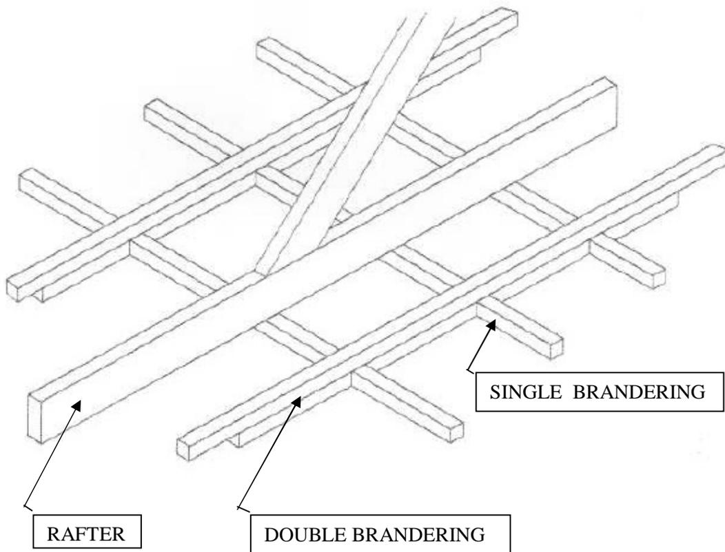
The “**double brandering**” will thus be running parallel to the main roof trusses normally and will rest on top of the single ones that are nailed (or even better screwed) to the main roof trusses.
